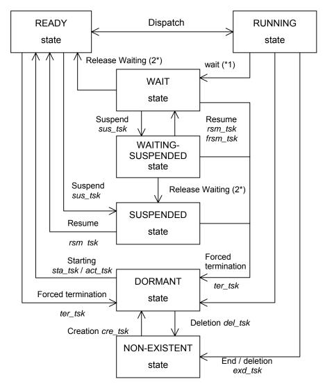
(\*1) slp\_tsk, tslp\_tsk,wai\_sem, twai\_sem, wai\_flg, twai\_flg, rcv\_mbx, trcv\_mbx, rcv\_mbf, trcv\_mbf, snd\_mbf, tsnd\_mbf, cal\_por, tcal\_por, acp\_por, tacp\_por, get\_mpl, tget\_mpl, get\_mpf, tget\_mpf, dly\_tsk, snd\_dtq, tsnd\_dtq, rcv\_dtq, trcv\_dtq, loc\_mtx, tloc\_mtx
